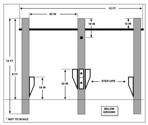
Figure B-3. Climbing bar dimensions, side view
