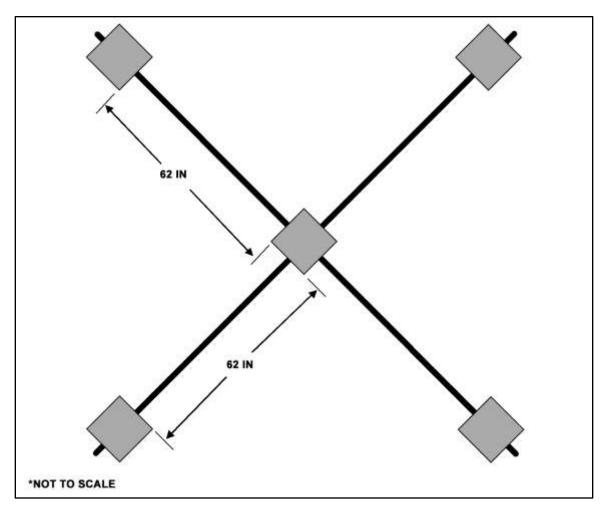
Figure B-2. Climbing bars, dimensions, top view
